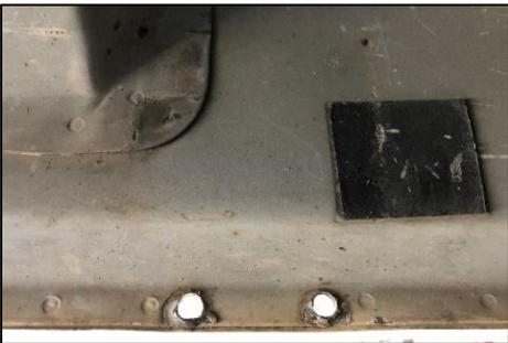
**Step 6:** Starting with the center bracket, install two 5/16" x 1" carriage bolts through the drilled holes and through the bracket. Use the 5/16" hex nuts and washers and hand tighten. Repeat for front and rear bracket.
